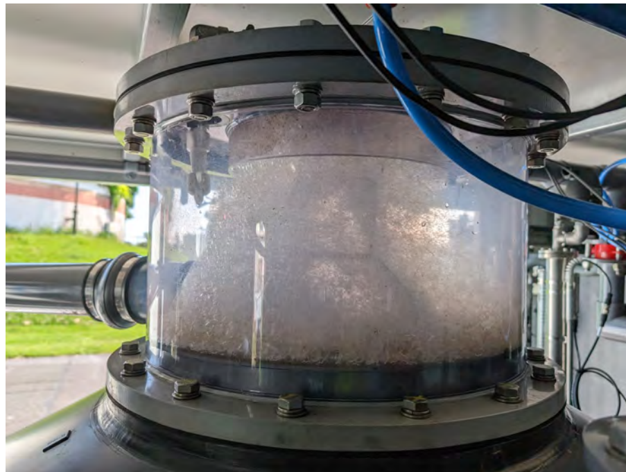
PFAS accumulate in concentrate at the top of the vessel
