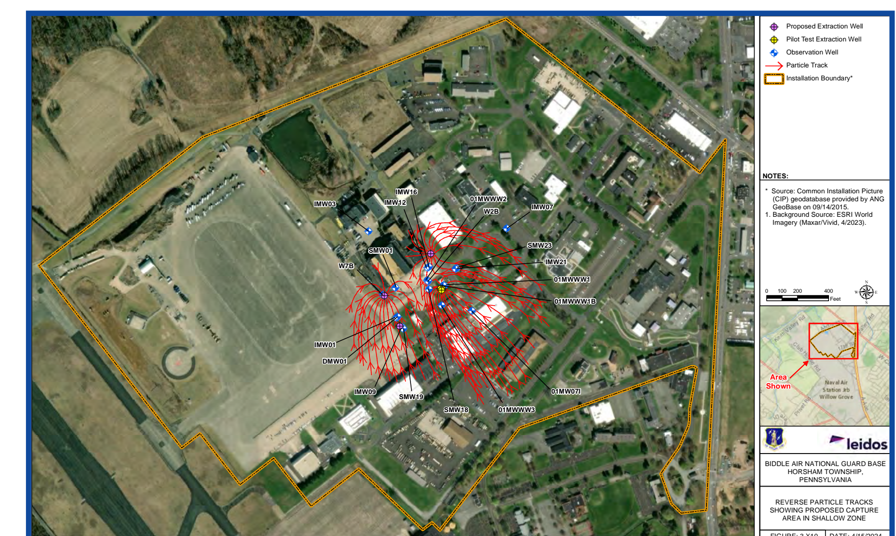
Figure showing location of existing extraction wells in pilot test plus three additional extraction wells and backward particle tracking to show upgradient capture zone.
